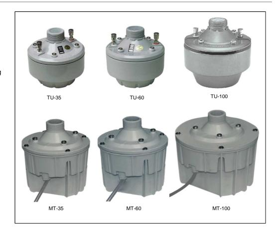
The driver units of the TU and MT Series are dedicated to be coupled with SHOW TH Series horn flares or to any device accepting 1 - 3/8" 18 male thread. Made of die cast aluminum for the TU Series and Plastic base/ Aluminum cover for the MT Series, the drivers deliver high SPL for public address applications.
